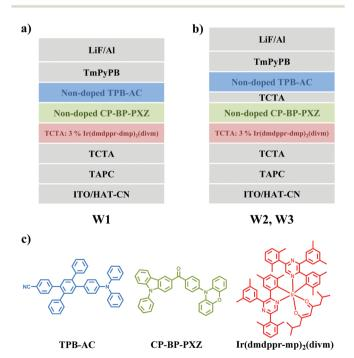
Fig. 1 (a) Structure diagram of the designed device W1 without an interlayer. (b) Structure diagram of the designed device W2 with a TCTA interlayer. (c) Chemical structures of TPB-AC, CP-BP-PXZ, and Ir(dmppr-mp)<sub>2</sub>(divm).
