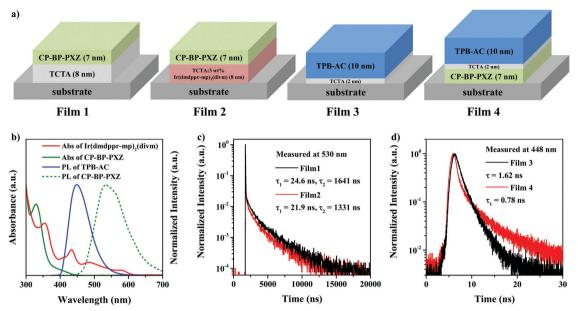
Fig. 4 (a) Structures of films 1-4. (b) Absorption spectra of the Ir(dmppr-mp)<sub>2</sub>(divm) and CP-BP-PXZ films, and PL spectra of the CP-BP-PXZ and TPB-AC films. (c) Transient PL spectra of films 1 and 2 measured at 530 nm. (d) Transient PL spectra of films 3 and 4 measured at 448 nm.
