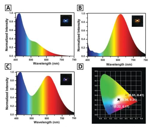
Fig. 10 Emission spectra of monochrome down-conversion LEDs fabricated by using (A) blue emitting Cu NCs and (B) orange emitting Cu NCs. Panel (C) shows an emission spectrum of the WLED fabricated by a combination of these two kinds of Cu NCs. Insets in (A-C) provide photographs of operating blue, orange and white LEDs; while panel (D) shows CIE coordinates of three respective LEDs. Reproduced with permission from ref. 101, Copyright 2016, Wiley-VCH
