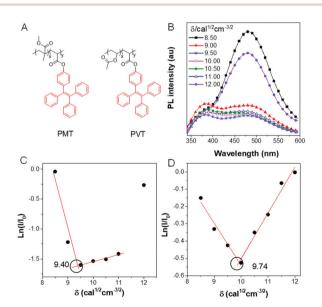
Fig. 11 (A) Chemical structure of PMT and PVT. (B) PL intensity of PMT in solvents with different solubility parameters. Plots of  $ln(I/I_0)$  of (C) PMT and (D) PVT to confirm the solubility parameter. Reproduced from ref. 73 with permission from MDPI journals.
