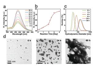
Fig. 2 Redox-responsive properties of TCSC bioprobes. (a) FL spectrum of TCSC after different incubation periods in 10 mM DTT; (b) FL intensity changes of TCSC bioprobes incubated in 10 mM DTT over time: (c) hydrodynamic diameter distribution changes of TCSC after different reaction times in 10 mM DTT; (d) TEM images of the corresponding nanoparticles after different incubation periods.
