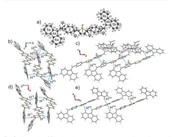
Fig. 2 X-ray data: (a) molecular structure, atom and cycle numbering of BFMPT, (b) and (c) crystal structure and intermolecular interactions in form I, (d) and (e) crystal structure and intermolecular interactions in form II. Dashed blue lines represent noncovalent interactions.
