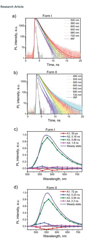
Fig. 5 PL kinetics of BFMPT polymorphs: PL time profiles recorded using form I (a) and form II (b) over the whole emission band after the excitation at 375 nm; the solid lines represent 4-exponential fits convoluted with the instrument response function (IRF); decay associated spectra obtained from 4 exponential fits of fluorescence time profiles for form I (c) and form II (d) in comparison with steady-state spectra recorded using 375 nm laser excitation.
