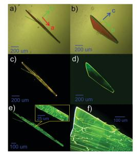
Fig. 1 Optical images of BFMPT single crystals. In transmitted light: form I (a) and form II (b); under blue laser irradiation (405 nm): form I (c) and form II (d), (e) form I after heating at 280 °C for 5 seconds and (f) form II after heating at 280 °C for 5 seconds.
