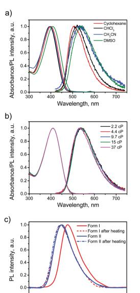
Fig. 4 Steady-state optical data: absorption and PL spectra of BFMPT in different organic solvents (a) and DMSO:glycerol mixtures of different viscosity (2.2-37 cP) (b); PL spectra of BFMPT crystals measured by integrating sphere (c): form I before (red) and after heating at 280 °C (dashed red); form I before (blue) and after heating at 280 °C (dashed blue).
