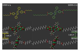
Fig. 8 Calculated electron distributions of HOMOs-LUMOs and the energy levels of TPPP-C6 (left) and TPPP-C12 (right).
