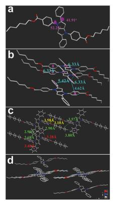
Fig. 7 The crystal structure (a), intermolecular interactions (b and c), and packing patterns (d) of TPPP-C6. Green and red lines represent the interand intramolecular  $C-H\cdots\pi$  interactions, respectively, and yellow lines represent the C-H···O interactions in Fig. 8(c).
