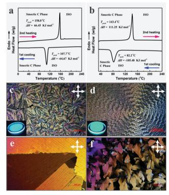
Fig. 4 DSC curves of TPPP-C6 (a) and TPPP-C12 (b) recorded under nitrogen during the first cooling and second heating cycles with a scan rate of 5 °C min $^{-1}$ . Mesomorphic textures observed on cooling TPPP-C6 (c) to 103 °C and TPPP-C12 (d) to 87 °C at a cooling rate of 0.5 °C min $^{-1}$ , the inset emission photos of the LC phase taken under UV light. POM patterns of TPPP-C6 (e) and TPPP-C12 (f) in the crystalline phase with a faster cooling rate of over 5 °C min $^{-1}$ .
