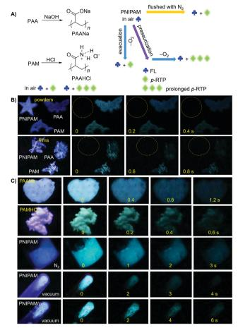
Fig. 3 (A) Schematic illustration of the modulation of p-RTP properties of different polymers. (B and C) Photographs of different powders and films taken under 312 nm UV light or after ceasing the UV irradiation at ambient conditions, under nitrogen or in vacuum. PNIPAM/p: pressed PNIPAM powders under a pressure of 2000 kg cm<sup>-2</sup> for 1 min.
