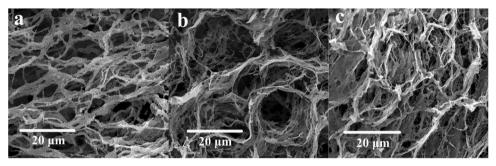
Fig. 3 SEM analysis of the copolymer in deionized water: (a) HPAM, magnified 2000 times; (b) Poly-A, magnified 2000 times; (c) Poly-B, magnified 2000 times (copolymer concentration, 2000 mg L<sup>-1</sup>).
