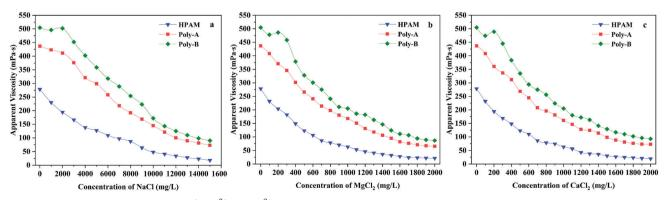
Fig. 8 Salt resistance of copolymers for Na<sup>+</sup>, Mg<sup>2+</sup> and Ca<sup>2+</sup>.
