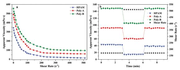
(a) Shear thinning behavior of the copolymers and (b) shear recovery of the copolymers.
