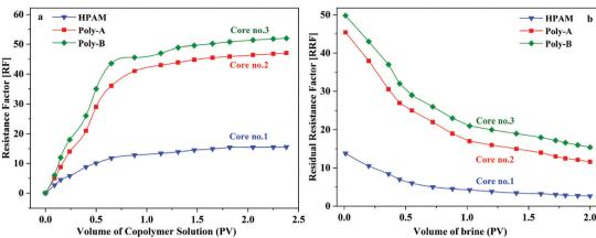
Flow behavior of copolymer solutions in porous media (copolymer concentration, 2000 mg  $L^{-1}$ ; 70 °C).
