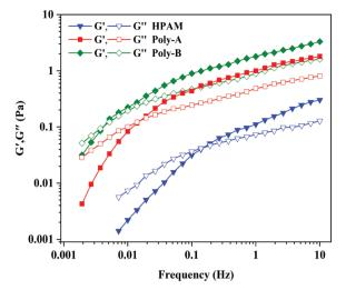
Fig. 9 Viscoelastic behavior of copolymers.
