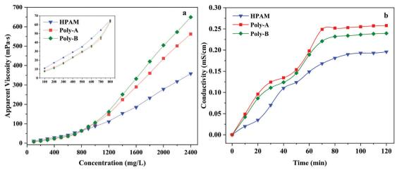
(a) Tackifying of copolymers and (b) the dissolution time curves of copolymers
