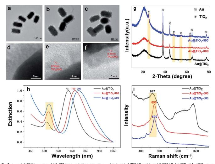
Fig. 3 (a and d) TEM images and HR-TEM images before annealing and at (b and e) 300 °C and (c and f) 500 °C. (g) XRD of Au@TiO<sub>2</sub> nanostructures before and after annealing. (h) UV-visible spectroscopy of Au@TiO2 nanostructures before and after annealing. (i) Raman spectroscopy of Au@TiO2 nanostructures before and after annealing
