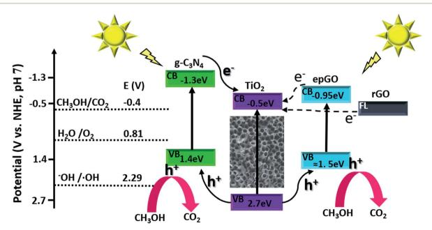
Scheme 1 Energy diagram and schematic illustration of charge transfer in q-C<sub>3</sub>N<sub>4</sub> and graphene coatings on TiO<sub>2</sub>NTs.
