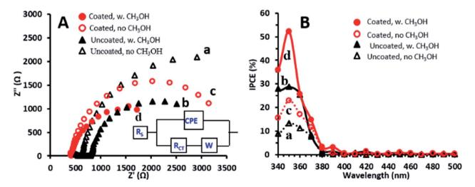
Fig. 3 (A) EIS Nyquist plots for  $TiO_2NTs$  (a and b) and  $TiO_2NTs/g-C_3N_4$  (c and d) in the absence and presence of 1 M methanol. Inset: equivalent circuit. (B) IPCE spectra at a bias of +0.4 V for TiO<sub>2</sub>NTs (a and b) and TiO<sub>2</sub>NTs/g-C<sub>3</sub>N<sub>4</sub> (c and d) in the absence and presence of methanol.
