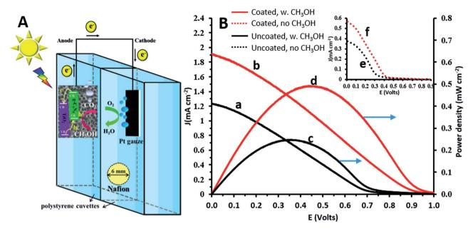
Fig. 4 (A) Schematic illustration of a photofuelcell based on the  $TiO_2NTs/g-C_3N_4$  photoanode. (B) Current density (a and b) and power density (c and d) vs. voltage curves for the photofuelcell with  $TiO_2NTs$  and  $TiO_2NTs/g-C_3N_4$  in 0.1 M  $Na_2CO_3$  and 1 M methanol. Inset: current density vs. voltage curves under the same operating conditions without methanol for  $TiO_2NTs$  (e) and  $TiO_2NTs/g-C_3N_4$  (f).
