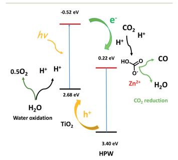
Fig. 10 Elementary steps in the CO<sub>2</sub> photocatalytic reduction to CO. Band levels versus NHE.34
