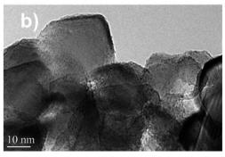
Fig. 7 TEM images of the calcined (a) and used (b) Zn-HPW/TiO<sub>2</sub> catalyst.
