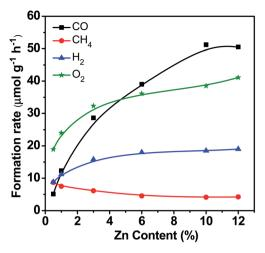
Fig. 3 CO, CH<sub>4</sub>, H<sub>2</sub> and O<sub>2</sub> formation rates over Zn-HPW/TiO<sub>2</sub> catalysts with different Zn loadings. Reaction conditions: catalyst, 0.1 g; gas phase pressure, CO<sub>2</sub> 0.2 MPa; H<sub>2</sub>O, 15 mL; irradiation time, 6 h.
