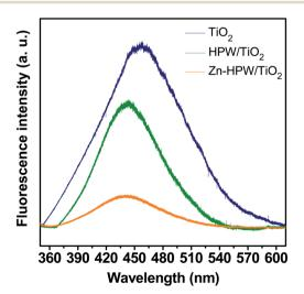
Fig. 5 Photoluminescence spectra of TiO<sub>2</sub>, HPW and Zn containing catalysts.
