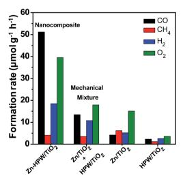
Fig. 4 CO, CH<sub>4</sub>, H<sub>2</sub> and O<sub>2</sub> formation rates over Zn-HPW/TiO<sub>2</sub>, Zn/ TiO<sub>2</sub>, HPW/TiO<sub>2</sub> and a mechanical mixture of Zn/TiO<sub>2</sub> + HPW/TiO<sub>2</sub> in the photocatalytic CO<sub>2</sub> reduction. Reaction conditions: catalyst, 0.1 g; gas phase pressure, CO<sub>2</sub> 0.2 MPa; H<sub>2</sub>O, 15 mL; irradiation time, 6 h.
