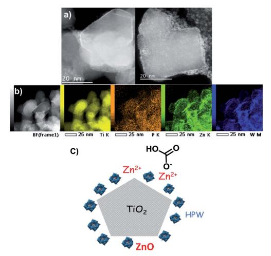
Fig. 8 (a) HAADF-STEM micrographs, (b) STEM-EDX elemental maps of Zn-HPW/TiO<sub>2</sub> catalyst and (c) a diagram of the Zn-HPW/TiO<sub>2</sub> catalyst structure.
