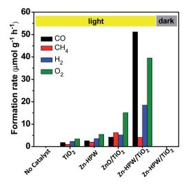
Fig. 2 CO, CH<sub>4</sub>, H<sub>2</sub> and O<sub>2</sub> formation rates over  $TiO_2$ , HPW and Zn containing catalysts in the photocatalytic reduction of  $CO_2$  in water. Reaction conditions: catalyst, 0.1 g; gas phase pressure,  $CO_2$  0.2 MPa; H<sub>2</sub>O, 15 mL; irradiation time, 6 h.
