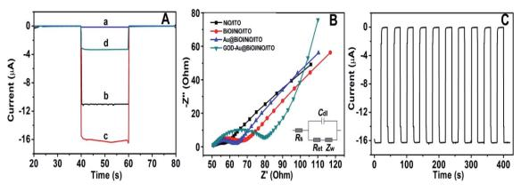
Fig. 6 (A) Photocurrent performance of (a) NiO/ITO (b) BiOI/NiO/ITO (c) Au@BiOI/NiO/ITO (d) GOD-Au@BiOI/NiO/ITO; the applied voltage is 0 V. (B) The corresponding EIS Nyquist plots (inset is the randles equivalent circuit of EIS). (C) PEC responses of the Au@BiOI/NiO/ITO electrode under several "on-off-on" irradiation cycles for 420 s (the applied voltage is 0 V).
