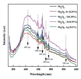
Fig. 5 PL spectra of the doped and pristine Nb<sub>2</sub>O<sub>5</sub>.
