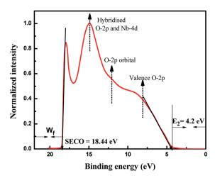
Fig. 4 UPS spectra of Nb<sub>2</sub>O<sub>5</sub>
