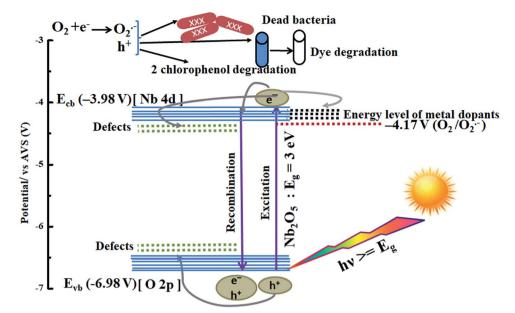
Fig. 15 Photocatalysis mechanism in metal-doped Nb<sub>2</sub>O<sub>5</sub>
