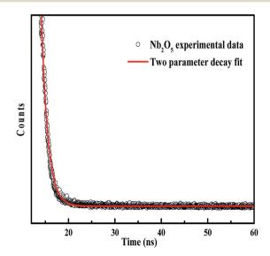
Fig. 6 TRF decay curve of Nb<sub>2</sub>O<sub>5</sub>.
