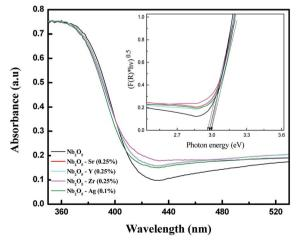
Fig. 3 UV-vis absorbance spectra of pristine and doped Nb<sub>2</sub>O<sub>5</sub> and the inset presents the transformed Kubelka-Munk function vs. photon energy.
