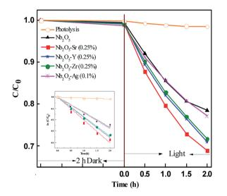
Fig. 9 Effect of dopants in  ${\rm Nb_2O_5}$  for OG degradation and the inset presents rate kinetics.
