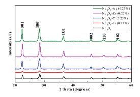
Fig. 1 XRD patterns of Nb<sub>2</sub>O<sub>5</sub> doped with Sr, Y, Zr, and Ag of 0.25 atom%.
