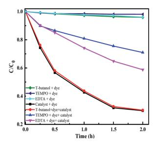
Fig. 14 Radical trapping experiment with scavengers and MB as the pollutant.
