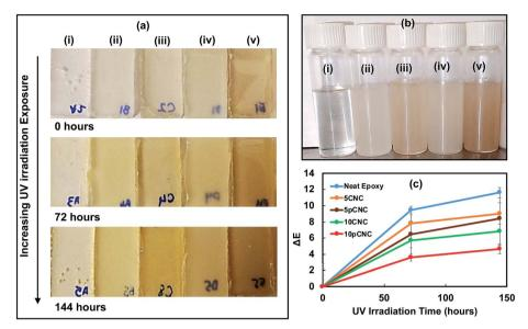
Fig. 8 (a) Epoxy nanocomposites cured and UV irradiated for 0, 72 and 144 hours; (b) epoxy nanocomposites before curing: (i) neat epoxy, (ii) 5CNC, (iii) 5pCNC, (iv)10CNC and (v) 10pCNC, respectively; (c) color change related to samples.
