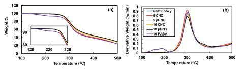
Fig. 10 TGA analysis of epoxy nanocomposites with different fillers. (a) Weight loss curve and (b) weight loss derivative curve
