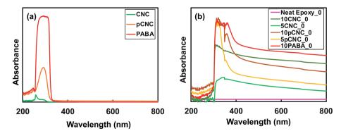
Fig. 5 Comparative UV absorbance of (a) CNCs, PABA and pCNC; (b) epoxy nanocomposites prior to UV irradiation.
