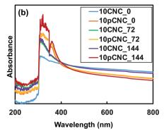
Fig. 6 Effect of UV irradiation on the UV absorption of (a) epoxy nanocomposites with 5 wt% CNCs and pCNC after UV irradiation for 0, 72, and 144 hours; (b) epoxy nanocomposites with 10 wt% CNCs and pCNC after UV irradiation for 0, 72, and 144 hours.
