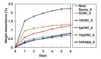
Fig. 11 Water absorption of composite specimens prior to UV exposure.
