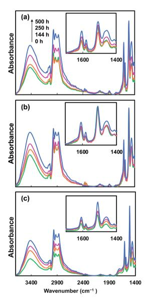
Fig. 7 FTIR spectra of (a) neat epoxy, (b) 10CNC and (c) 10pCNC upon UV degradation.
