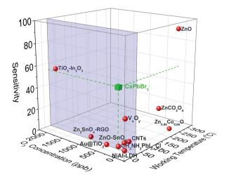
Fig. 3 Sensitivity vs. O<sub>3</sub> concentration and working temperature for the sensing elements found in the literature. The blue frame indicates the room temperature regime.
