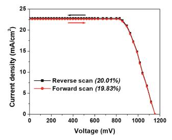
Fig. 5 J-V plot (both in reverse and forward scans) for the best performing PSCs with 3D hierarchical SnO<sub>2</sub> nanospheres showing their hysteresis-free behavior.
