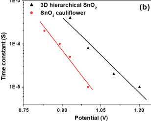
Fig. 8 (a) Steady-state PL spectra of perovskites on different  $SnO_2$  nanostructures and (b) electron lifetime for the perovskites based on different  $SnO_2$  nanostructures.
