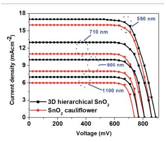
Fig. 3  $\,$   $\it J-V$  curves as a function of the ETL thickness for two distinct  $\rm SnO_2$  nanostructures.
