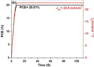
Fig. 4 (a) J-V plot (reverse scan) for the best performing PSCs with 3D hierarchical  $SnO_2$  nanospheres and (b) the steady state efficiency of the corresponding devices measured at maximum power output.
