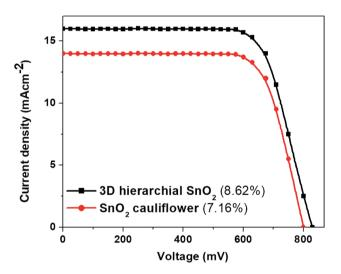
Fig. 6 Comparison of J-V curves of DSSCs fabricated with two distinct SnO2 nanostructures.
