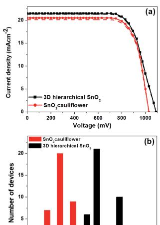
Fig. 2 (a) Comparison of J-V curves of PSCs based on two distinct SnO<sub>2</sub> nanostructures and (b) histograms of the corresponding PSCs showing variations in the PCE for 45 individual cells for each nanostructure.
