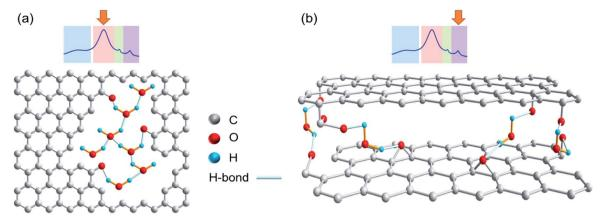
Fig. 4 Chemical structures showing different water types present in the remotely photo-oxidized sample CB<sub>R72</sub>. (a) Intralayer or pore water. (b) Interlayer water.
