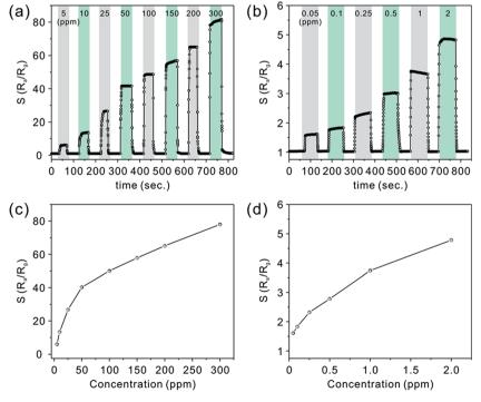
Fig. 6 (a and b) The real-time response curves of CZ-3 porous nanobelts toward different concentrations of acetone at the optimal working  $temperature\ of\ 325\ ^\circ\text{C}, and\ (c\ and\ d)\ the\ relationship\ between\ the\ relative\ response\ and\ the\ concentration\ of\ acetone\ for\ CZ-3\ porous\ nanobelts$ at the optimal working temperature of 325 °C.
