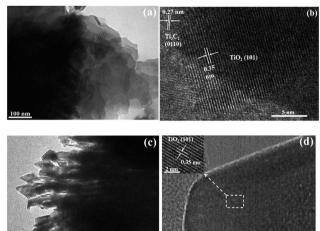
Fig. 4 HRTEM images of (a and b) TOH and (c and d) TF samples.
