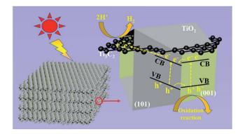
Fig. 6 Schematic of the tentative photocatalytic mechanism of truncated octahedral bipyramidal  $\text{TiO}_2/\text{Ti}_3\text{C}_2$  hybrids under light irradiation.
