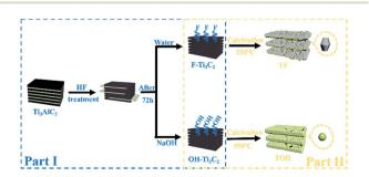
Fig. 1 Schematic of the preparation procedure for the synthesis of MXene  ${\rm Ti}_3{\rm C}_2/{\rm Ti}{\rm O}_2$  composite photocatalysts.
