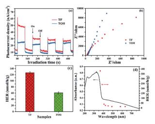
Fig. 5 (a) Photocurrent responses and (b) EIS patterns of TF and TOH samples. (c) Hydrogen evolution rate (HER) of the samples under 1 h light irradiation using glycerinum/water (1:10 vol%) solution as a sacrificial agent and (d) wavelength-dependent HER of TF under 1 h monochromatic light irradiation by using glycerinum/water (1:10 vol%) solution as a sacrificial agent.
