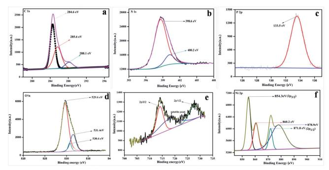
XPS spectra for 20 wt% NFO/PCN in the regions of: (a) C 1s, (b) N 1s, (c) P 2p, (d) O 1s, (e) Fe 2p and Ni 2p.
