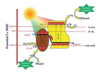
Scheme 3 Schematic presentation of the degradation of phenol and evolution of H<sub>2</sub> over 20 wt% NFO@P-CN.
