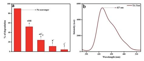
Fig. 13 (a) Percentage degradation of phenol over 20 wt% NFO@P-CN in the presence of scavenging agents, (b) confirmation of \*OH generation in 20 wt% NFO@P-CN through the TA test.
