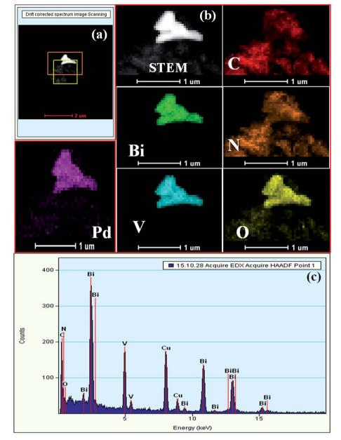
Fig. 4 (a) HAADF and (b) STEM-HAADF images of individual elements, and (c) EDAX spectrum of (Pd3%)/SBVCN-37.
