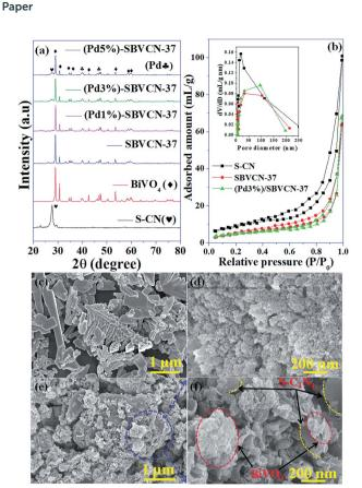
Fig. 1 (a) Powder XRD patterns of all the materials synthesized in this study, (b) N<sub>2</sub> adsorption-desorption isotherms of S-CN, SBVCN-37, and (Pd3%)/SBVCN-37, (inset shows BJH pore size distribution) and FESEM images of (c) BiVO<sub>4</sub>, (d) S-CN, (e) SBVCN-37, and (f) (Pd3%)/ SBVCN-37 photocatalyst.
