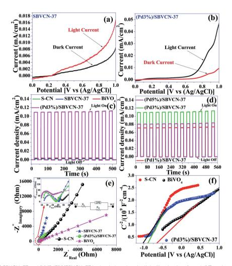
Fig. 7 LSV curves of (a) SBVCN-37 and (b) (Pd3%)/SBVCN-37 in the dark and under light illumination. (c and d) Transient photocurrent (i-t) of all the photocatalysts, (e) EIS profiles (inset shows enlarged profiles at the low frequency region and simulated equivalent circuit), and (f) Mott-Schottky plots of BiVO<sub>4</sub>, S-CN, and (Pd3%)/SBVCN-37 at the constant frequency of 1000 Hz.
