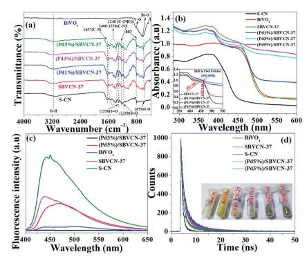
Fig. 5 (a) FTIR spectra, (b) DRUV-visible spectra, (c) Steady-state photoluminescence spectra, and (d) time-resolved spectra of the materials investigated in this study (inset shows a photograph of the synthesized powder photocatalysts).
