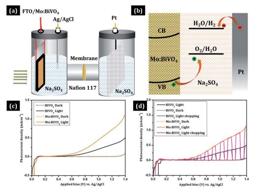
Fig. 7 (a) Experimental set-up of an H-shaped photoelectrochemical cell with two separate compartments for photocatalytic oxidation of water to O<sub>2</sub>; (b) mechanism of photoelectrochemical water splitting; (c) photocurrent density-potential curves recorded under dark (dotted line) and light (solid line) (scan rate =  $10 \text{ mV s}^{-1}$ ); (d) chopping performance.
