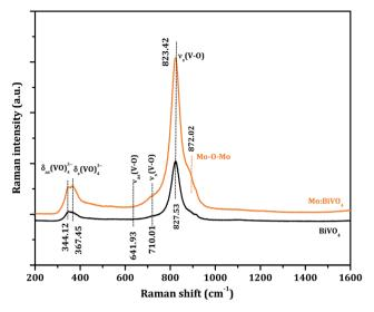
Fig. 4 Raman spectra of BiVO<sub>4</sub> and Mo:BiVO<sub>4</sub> nanoporous thin films.
