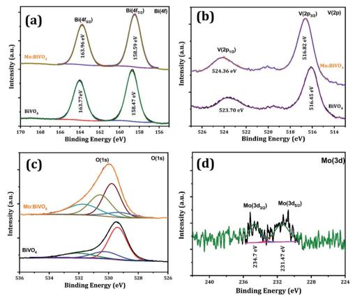
Fig. 6 XPS spectra of pristine BiVO<sub>4</sub> and Mo:BiVO<sub>4</sub> thin films; high-resolution core level XPS spectrum of (a) Bi 4f (b), V 2p (c), O 1s (d) and Mo 3d.
