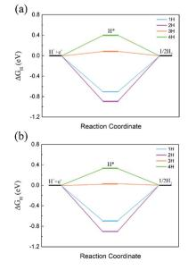
Fig. 6  $\Delta G_H$  with different hydrogen coverages on the  $C_2N$  layer in (a)  $C_2N/GaTe$  and (b)  $C_2N/InTe$  heterojunctions.
