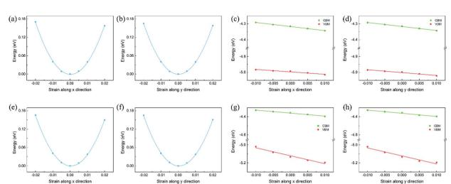
Fig. 5 The relationship between energy and strain for (a, b)  $C_2N/GaTe$  and (e, f)  $C_2N/InTe$ . The CBM and VBM along the x and y directions as a function of deformation proportion for (c, d)  $C_2N/GaTe$  and (q, h)  $C_2N/InTe$ .
