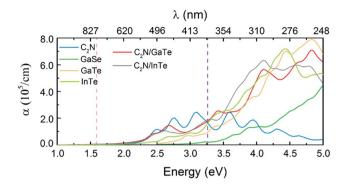
Fig. 4 Optical absorption coefficients for the isolated C2N, GaSe, GaTe, and InTe monolayers as well as C2N/GaTe and C2N/InTe heterojunctions. The area between the red and the purple lines represents the visible-light range.
