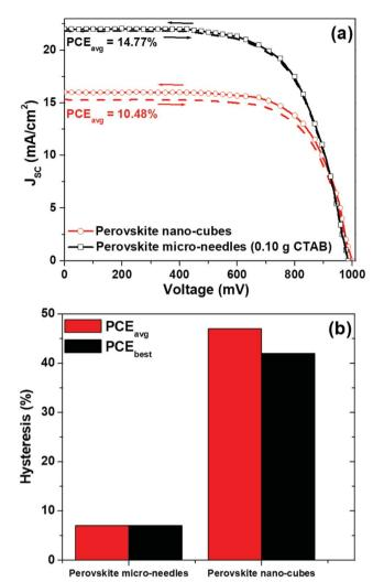
Fig. 4 (a) Comparison of J-V plots of perovskite devices based on MAPbl<sub>3</sub> micro-needles and nano-cubes, and (b) hysteresis for devices with MAPbI<sub>3</sub> micro-needles and nano-cubes, respectively
