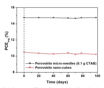
Fig. 6 Long-term stability test of un-encapsulated devices based on MAPbI $_3$  micro-needles and perovskite nano-cubes stored in dry air.
