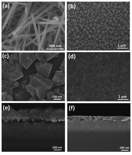
Fig. 2 Plane-view SEM micrographs showing (a) a magnified view of Pbl<sub>2</sub> micro-needles and (b) nano-cubes of the perovskite, (c) a magnified view of perovskite nano-cubes and (d) MAPbl<sub>3</sub> micro-needles, and cross-sectional SEM images of FTO glass substrate/ZnO compact layer/(e) perovskite nano-cubes and (f) MAPbl<sub>3</sub> micro-needles, respectively.
