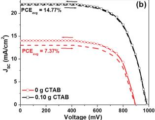
Fig. 3 Typical J-V plots of various micro-needle perovskite solar cells (a) as a function of CTAB concentration (in the reverse direction only), and (b) based on 0 g and 0.1 g CTAB concentration, in different scanning directions, respectively.
