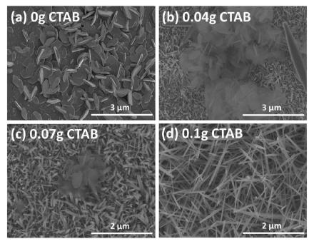
Fig. 1 Plane-view SEM micrographs of the  $Pbl_2$  micro-needles synthesized by the hydrothermal route with various amounts of CTAB: 0 g (a), 0.04 g (b), 0.07 g (c), and 0.10 g (d), respectively.
