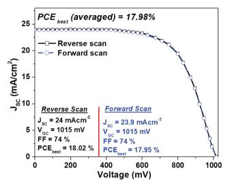
Fig. 5 J-V curves (both in the forward and reverse scans) for the best-performing device with MAPbl<sub>3</sub> micro-needles.
