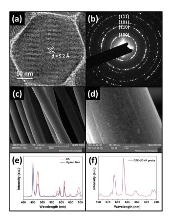
**Fig. 2** (a) HRTEM and (b) SAED images of the core@shell UCNPs. SEM images of (c) CFC and (d) the CFC-UCNP probe. UCL spectra of (e) OA-capped and ligand free core@shell UCNPs and (f) the CFC-UCNP probe under 980 nm excitation.
