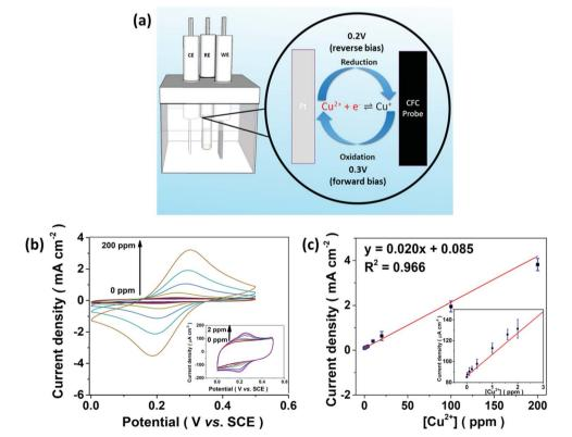
Fig. 4 (a) A diagram illustrating the E-chem processes on the CFC-UCNP probe. (b) CV curves of the CFC-UCNP probe in response to 0-200 ppm  $Cu^{2+}$  ions recorded within the potential window of 0-0.5 V at 100 mV s<sup>-1</sup>. (c) The linear relationship between the E-chem signals and  $[Cu^{2+}]$  obtained at 0.3 V. The insets are the enlarged plots for 0-2 ppm  $Cu^{2+}$  ions.
