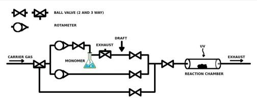
Fig. 1 The experimental reactor line setup.
