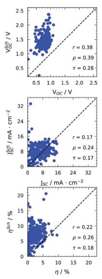
Fig. 1 Comparison between computed and experimental photovoltaic properties
