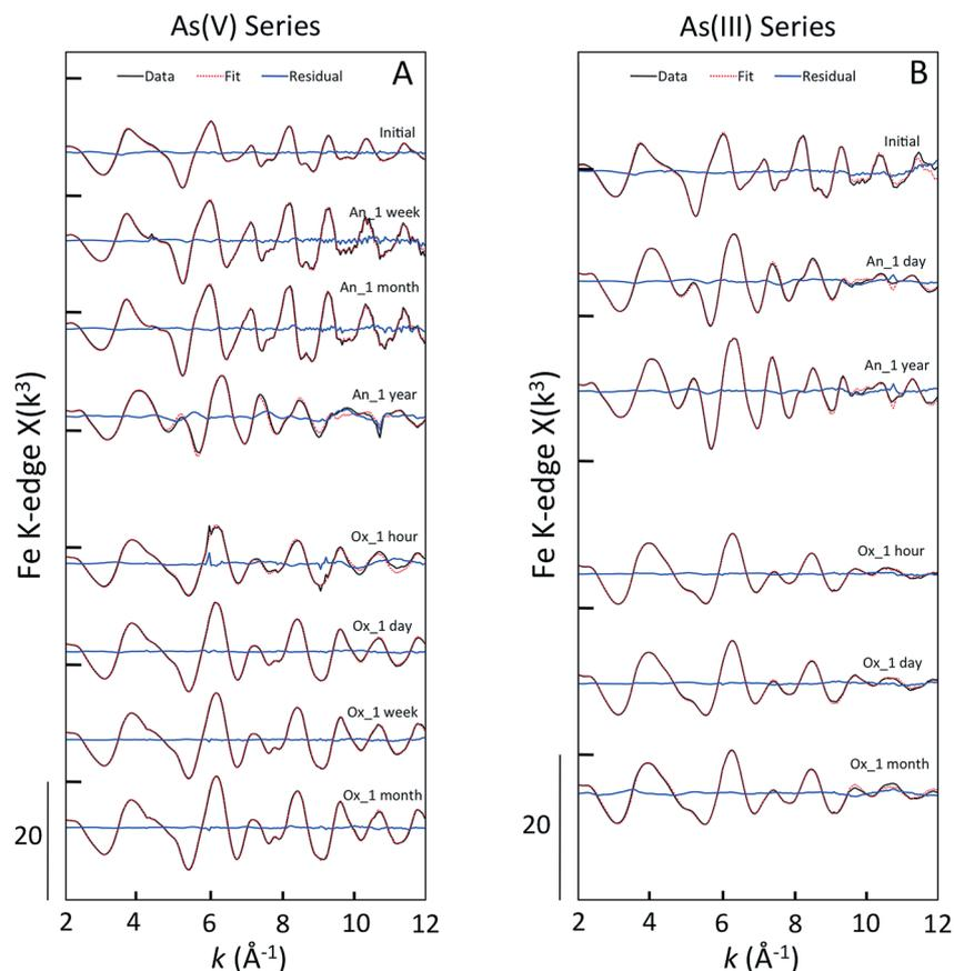
Fig. 2 Fe K-edge EXAFS spectra of green rust aging samples in As(v) experiments (left panel) and As(III) experiments (right panel). The ITFA fitting output is shown in dotted red lines and the data is given in solid black lines. The fitting residual is given in solid blue lines. The anaerobic aging series (e.g. An\_1 week) are given above the oxic aging samples (e.g. Ox\_1 hour).
