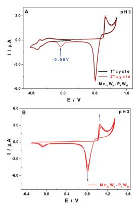
Fig. 5 CVs of  $Mn_{10}W_4-P_8W_{48}$  in 0.5 M Li<sub>2</sub>SO<sub>4</sub> + H<sub>2</sub>SO<sub>4</sub> at pH 3.0. POM concentration: 0.07 mM. (A) Potential range was between 1.35 V and -0.82 V. The scan was started at +0.2 V towards the negative potentials. (B) Potential range was between 1.35 V and -0.30 V. The scan was started at +0.2 V towards the positive potentials. Working electrode: EPG; counter electrode: Pt wire; and reference electrode: SCE. Scan rate: 10 mV s<sup>-1</sup>.
