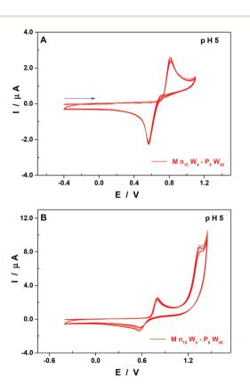
**Fig. 6** CVs of  $Mn_{10}W_4-P_8W_{48}$  in 1.0 M LiCH $_3$ CO $_2$  + CH $_3$ CO $_2$ H at pH 5.0. POM concentration: 0.07 mM. (A) Potential range was between 1.10 V and -0.40 V. The scan was started at +0.2 V towards the negative potentials. (B) Potential range was between 1.45 V and -0.40 V. The scan was started at +0.2 V towards the positive potentials. Working electrode: EPG; counter electrode: Pt wire; and reference electrode: SCE. Scan rate: 10 mV s $^{-1}$ .
