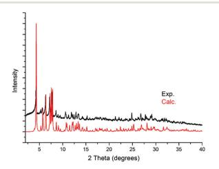
Fig. 4 Experimental powder diffraction pattern of  $KLiMn-Mn_{10}W_4-P_8W_{48}$  and the calculated powder diffraction pattern from the single-crystal X-ray diffraction structure of  $KLiMn-Mn_{10}W_4-P_8W_{48}$ .
