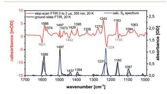
Fig. 13 FTIR ground state spectrum at 20 K (black), calculated  $S_0$  spectrum (B3LYP-D3(BJ)/def2-TZVP, FWHM = 8 cm<sup>-1</sup>, Gaussian profile, scaled by 0.975) (blue) and step-scan difference spectrum 0 to 2  $\mu$ s after excitation ( $\lambda_{EX}$  = 355 nm) (red) of Cu-2b.
