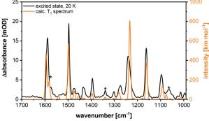
**Fig. 14** Excited state spectrum (black) and calculated  $T_1$  spectrum (orange) (B3LYP-D3(BJ)/def2-TZVP, FWHM = 8 cm<sup>-1</sup>, Gaussian profile, scaled by 0.975) of **Cu-2b**. The  $T_1$  specific bands are marked with asterisks.
