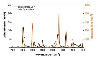
**Fig. 15** Excited state spectrum (black) and calculated  $T_1$  spectrum (B3LYP-D3(BJ)/def2-TZVP, FWHM = 8 cm $^{-1}$ , Gaussian profile, scaled by 0.975) (orange) of **Cu-1b**. The  $T_1$  specific bands are marked with asterisks.
