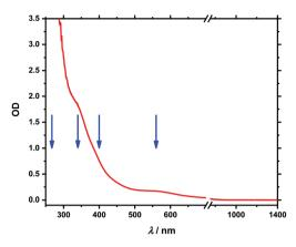
Fig. 2 Stationary absorption spectrum of  $Fe(CO)_2CpGe_9Hyp_3$  between 250 and 1400 nm. Blue arrows mark excitation wavelengths at 258/267, 340, 388/400 and 560 nm, respectively.
