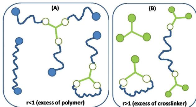
Fig. 5 Illustration of the most common sol structures for the two scenarios of (A) excess of polymer and (B) excess crosslinker. Networks resulting from  $r < 1$  possess by far the most complex dynamical behaviour, whereas those resulting from  $r > 1$  may be prone to curing over time when the utilised crosslinker is hydride-functional. Reproduced from ref. 14 with permission from the Technical University of Denmark (DTU), copyright 2017.
