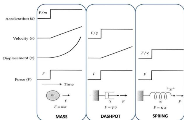
Fig. 6 The mechanical behaviour of a mass, a dashpot and a spring. The mechanical properties of elastomers can be modelled as a combination of these three elements. In the ideal case, these mechanical properties arise solely from an entropic spring contribution. Reproduced from ref. 14 with permission from the Technical University of Denmark (DTU), copyright 2017.
