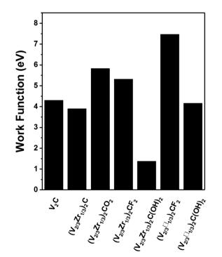
Fig. 5 Work functions of V<sub>2</sub>C, pristine (V<sub>2/3</sub>Zr<sub>1/3</sub>)<sub>2</sub>C, bimetallic (V<sub>2/3</sub>Zr<sub>1/3</sub>)<sub>2</sub>CX<sub>2</sub> and vacancy-ordered (V<sub>2/3</sub> $\square_{1/3}$ )<sub>2</sub>CX<sub>2</sub> MXenes.
