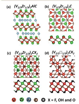
Fig. 1 Structures of parent MAX phase  $(V_{2/3}Zr_{1/3})_2AIC$  (a), pristine bimetallic MXene  $(V_{2/3}Zr_{1/3})_2C$  (b), functionalized bimetallic MXene  $(V_{2/3}Zr_{1/3})_2CX_2$  (c) and vacancy-ordered ( $V_{2/3}\square_{1/3}$ )<sub>2</sub>CX<sub>2</sub> (X = F, OH and O) MXene (d). The unit cell of MXenes is marked by a blue dotted line
