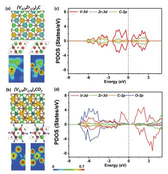
Fig. 2 Spin polarized charge densities and electron localization function (ELF) maps (perpendicular to [001] direction) are shown for  $(V_{2/3}Zr_{1/3})_2CF_2$  (a) and  $(V_{2/3}\square_{1/3})_2F_2$  (b), where spin up and spin down densities are shown in yellow and light blue, respectively. The units of color scale is "probability". Project density of states (PDOS) of  $(V_{2/3}Zr_{1/3})_2CF_2$  (c) and  $(V_{2/3}\Box_{1/3})_2F_2$  (d). Fermi level (black dotted line) is set to zero.
