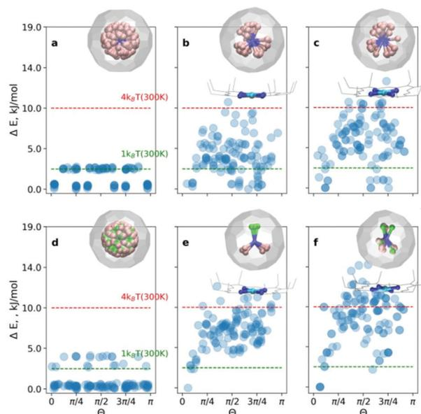
**Fig. 2** Relative energy distributions as a function of the order parameter  $\theta$  for (a and d) isolated  $\text{Sc}_3\text{N}@C_{80}$  and  $\text{YSc}_2\text{N}@C_{80}$ , (b and e) complex systems (**COS-0**, **COS-1**) and (c and f) crystal systems (**CRS-0**, **CRS-1**), respectively. The right upper corner graphics show superposed structures with  $\Delta E < 2.5 \text{ kJ mol}^{-1}$ .
