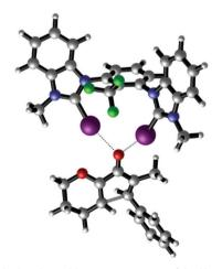
**Fig. 5** DFT-calculated transition state structure of the Nazarov cyclisation catalysed by halogen bond-donor **syn-9** (M06-2X D3 def2-TZVP(D)).<sup>25</sup> Selected distances [Å] and angles [°]: I–O 2.68 and 2.69; C–I–O 162 and 164. Graphic generated using CYLview.<sup>26</sup>
