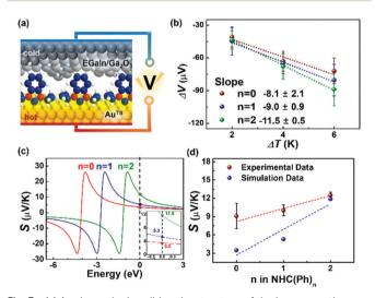
Fig. 3 (a) A schematic describing the structure of the large-area thermoelectric junction. (b) Plots of  $\Delta V$  as a function of  $\Delta T$ . (c) Simulations of S values based on the transmission function and Landauer formula (eqn (S2) and (S3) in the ESI†). The inset shows the magnification of Seebeck coefficient near the Fermi level of EGaln. (d) Plots of experimental and theoretical S values as a function of the molecular length.
