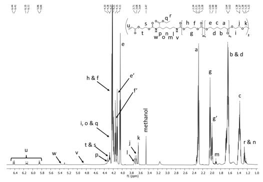
Fig. 1 <sup>1</sup>H NMR in CDCl<sub>3</sub> showing the characteristic peaks for CL, TMC, LDI, and acrylate protons in the final polymer. The PCTAc 50:50 copolymer is shown as a representative example.
