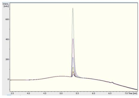
Fig. 3 (Upper) Calibration curve of MDMA between 1.5–50  $\mu g$  mL<sup>-1</sup>,  $R^2=0.9996$ , (lower) UV chromatogram MDMA RT = 5.4 min of the calibration curve concentrations.
