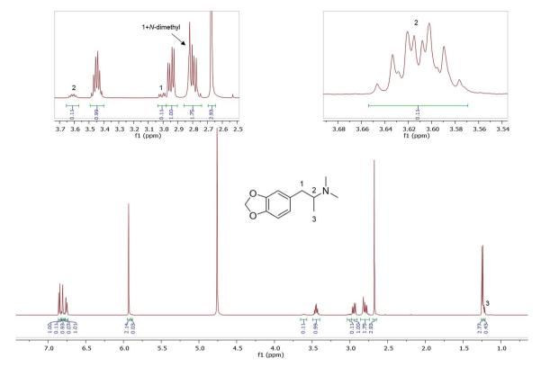
Fig. 5  $^{1}$ H NMR (in D<sub>2</sub>O) of sample HN165, MDMA containing MDDMA impurity with expansions revealing signals for MDDMA positions 1, 2 and N-dimethyl.
