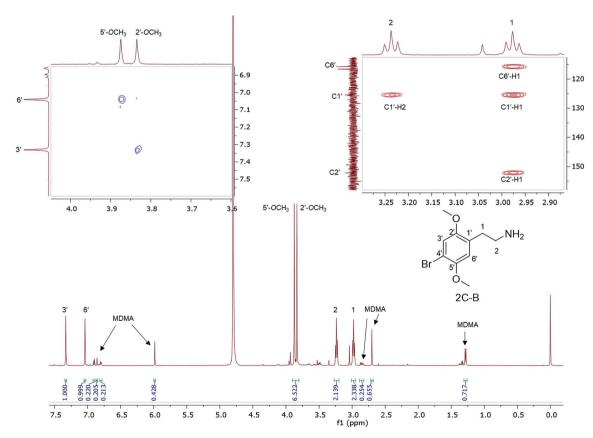
Fig. 6  $\,^{1}$ H NMR (in  $D_{2}$ O) of a 2C-B and MDMA mixture with TMSP 0.00 ppm, (top right) expansion of the HMBC spectra showing key HMBC connectivities, (top left) expansion of NOESY spectra revealing key NOE cross-peak connectivities.
