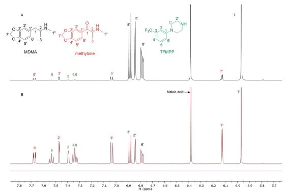
Fig. 1 Spectra of  $^{1}$ H NMR (in D<sub>2</sub>O) between 5.70–7.80 ppm of (A) sample HN157 and (B) sample HN153T, revealing significant differences in the ratio of each component.
