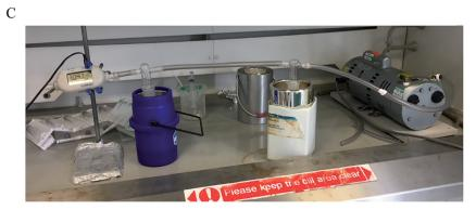
Fig. 2 In-house constructed SC smoking simulation model: (A) graphic, (B) cigarette inserted into the quartz tube, (C) Copley flow rate meter in position.
