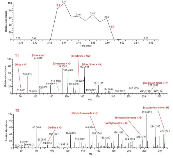
Mass spectra of fresh human urine, demonstrating the sequential ionisation from the beginning of the electrospray (T1, above) and the end of the electrospray (T2, below).
