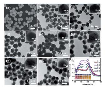
Fig. 2 (a) SEM image of Au NPs and (b-h) TEM images of the Au@Ag core—shell NPs synthesized under adding AgNO $_3$  in amounts from 0.50 to 3.50 mL at a gradient of 0.50 mL, respectively. The inset HRTEM images present the thickness of Ag shell from 1.0 to 10.0 nm; (i) the absorption spectra of Au NPs and Au@Ag core—shell NPs with the increase in the amount of AgNO $_3$  from 0.50 to 3.50 mL, the inset shows the colour of the solutions at different dosages of AgNO $_3$  solution.
