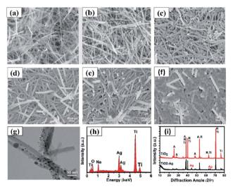
Fig. 5 SEM images of (a) TiO<sub>2</sub> NWs and Ag/TiO<sub>2</sub> NWs substrates prepared at different sputtering times: (b) 1, (c) 2, (d) 3, (e) 4, (f) 5 min; (g) TEM image of Ag/TiO2 NWs; (h) EDXS spectrum of Ag/TiO2 NWs substrate; (i) XRD spectra of TiO2 NWs and Ag/TiO2 NWs substrate (A, R, S, Ti and Ag represent anatase, rutile, sodium titanate, titanium and silver, respectively).
