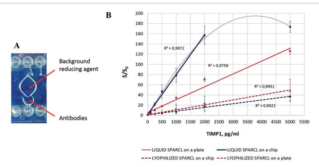
Fig. 4 The effect of the reagent lyophilization on the performance of the SPARCL<sup>TM</sup> assay. (A) Deposition of the lyophilized reagents on the chip. (B) Assay performance with liquid and lyophilized reagents (number of replicates n=3).
