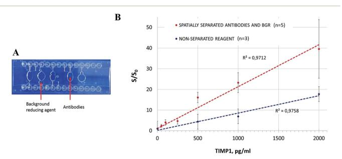
Fig. 5 Spatial separation of antibody mix and BGR on a chip. (A) Deposition of the lyophilized reagents on the chip. (B) Assay performance in comparison to non-separated reagent lyophilization ("incubation with BGR"). n -number of replicates.
