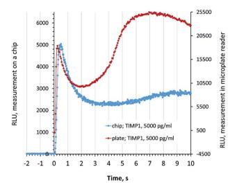
Fig. 2 Development of the luminescence in the chip luminometer and the microplate reader. RLU, relative light units. Zero time point corresponds to the injection of the trigger, the first peak (<1 s) indicates the SPARCL signal, and the slowly developing peak indicates the unspecific luminescence.
