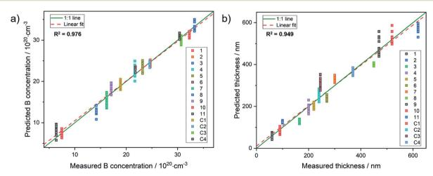
Fig. 4 Results from PLSR: (a) measured concentration vs. predicted values from the chemometric model and (b), predicted thickness vs. measured values for the diamond films.
