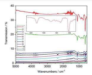
Fig. 2 IR-transmission spectra of the synthesised diamond films. Inset shows a zoomed view of sample 1 in the fingerprint region. (C1–C4 samples are left out due to the conductive silicon substrate used for these films, which completely absorbs the IR).
