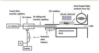
Fig. 1 Schematic figure of the LC-CPI-MS setup.
