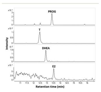
Fig. 4 SRM-chromatograms of E2, T, DHEA, and PROG from a standard mixture 10 ng mL<sup>-1</sup> using capillary LC-CPI-MS/MS.
