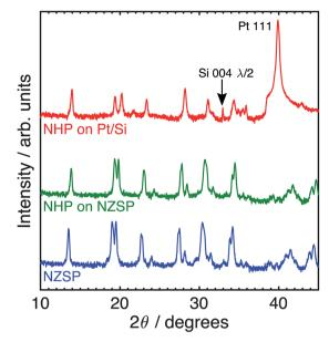
Fig. 4 Log-scale X-ray (Cu Kα) diffraction patterns of (top) NHP on platinized silicon (Pt/Si), (middle) NHP on an NZSP pellet, and (bottom) an as-received NZSP pellet
