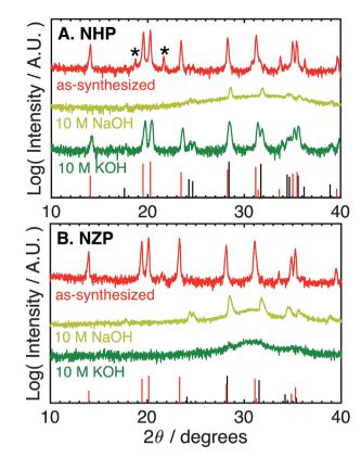
Fig. 1 Log-scale X-ray (Cu Kα) diffraction patterns of (A) NHP and (B) NZP powders as-synthesized and after aging for 72 h at 80 °C in different aqueous 10 M NaOH or KOH. Asterisks (\*) denote a slight HfP2O7 impurity. Red bars at the bottom of each plot denote PDFs for (A) NHP (04-002-2743) and (B) NZP (01-071-0959). Black bars denote PDFs for (A) HfO<sub>2</sub> (04-001-7440) and (B) ZrO<sub>2</sub> (04-002-8305).
