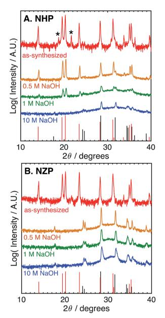
Fig. 3 Log-scale X-ray (Cu Kα) diffraction patterns of (A) NHP and (B) NZP powders before (virgin) after aging for 72 h at 80 °C in 0.5, 1, or 10 M aqueous NaOH. Asterisks (\*) denote a slight HfP<sub>2</sub>O<sub>7</sub> impurity. Red bars at the bottom of each plot denote PDFs for (A) NHP (04-002-2743) and (B) NZP (01-071-0959). Black bars denote PDFs for (A)  $HfO_2$ (04-001-7440) and (B) ZrO<sub>2</sub> (04-002-8305)
