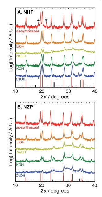
Fig. 2 Log-scale X-ray (Cu K $\alpha$ ) diffraction patterns of (A) NHP and (B) NZP powders as-synthesized and after aging for 72 h at 80 °C in varied 1 M basic aqueous electrolytes. Asterisks (\*) denote a slight HfP $_2$ O $_7$  impurity. Red bars at the bottom of each plot denote PDFs for (A) NHP (04-002-2743) and (B) NZP (01-071-0959). Black bars denote PDFs for (A) HfO $_2$  (04-001-7440) and (B) ZrO $_2$  (04-002-8305).
