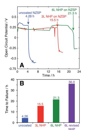
Fig. 7 (A) Open circuit potential as a function of time for uncoated and NHP-coated NZSP pellets with a silver back electrode immersed in 10 M KOH at 80  $^{\circ}$ C. (B) Comparison of lifetimes of NZSP pellets with various NHP coatings subjected to 10 M KOH at 80  $^{\circ}$ C.
