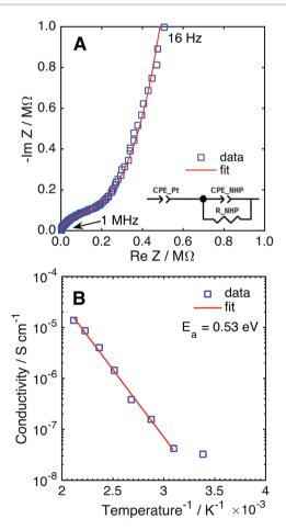
**Fig. 6** (A) Nyquist plot of NHP thin film in a Pt-NHP-Pt structure at 25 °C. (B) Na<sup>+</sup> conductivity of a NHP thin film as a function of temperature.
