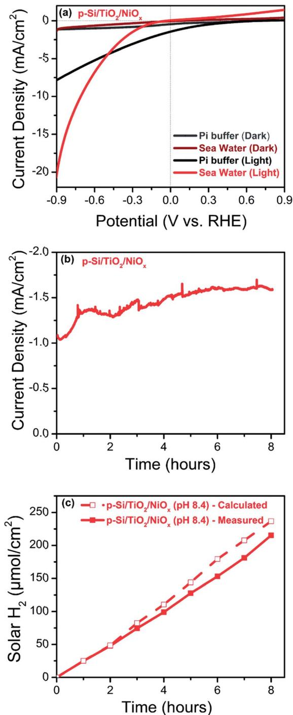
Fig. 8 Photo-electrochemical performance of the p-Si/TiO<sub>2</sub>/NiO<sub>x</sub> photoelectrode recorded under 1 sun illumination in artificial seawater at pH 8.4 (red) or pH 7.0 (black; 0.2 M phosphate buffer): (a) linear sweep voltammograms, (b) photo-current density measured at  $-0.3 V_{\text{RHE}}$  and (c) comparison of calculated (open squares) and measured (closed squares) photo generated hydrogen per geometric surface area of the photo-electrode at  $-0.3 V_{\text{RHE}}$  and 1 sun.
