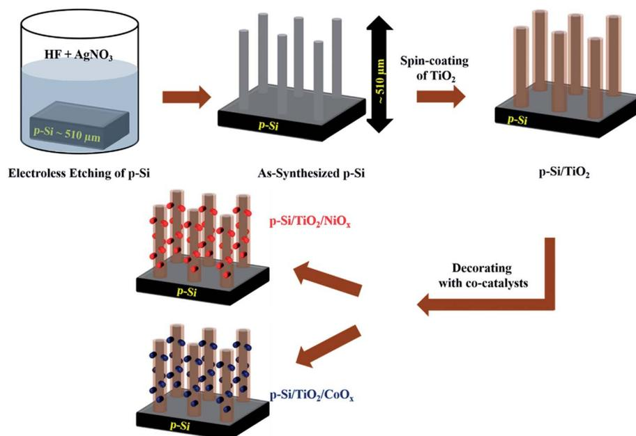
Fig. 1 Schematic representation (not to scale) of the preparation steps of p-Si micro-wires by wet-etching, their coating with TiO<sub>2</sub> and subsequent functionalization with NiO<sub>x</sub> or CoO<sub>x</sub> *via* spin coating and sintering. The procedure is described in detail in the ESI.†
