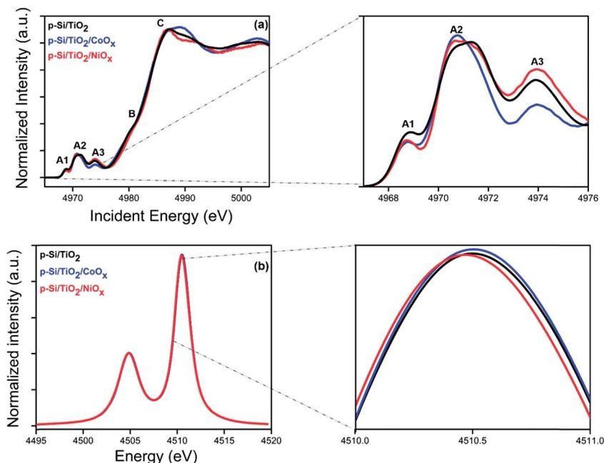
Fig. 7 X-ray spectroscopy characterization of p-Si/TiO<sub>2</sub> (black), p-Si/TiO<sub>2</sub>/CoO<sub>x</sub> (blue), p-Si/TiO<sub>2</sub>/NiO<sub>x</sub> (red): (a) HERFD-XANES spectra acquired at the Ti K-edge. The magnified view on the right shows the pre-edge peaks. (b) K $\alpha$  emission lines. The magnified view on the right shows the K $\alpha$  peak maximum.
