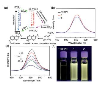
Fig. 4 (a) The ESIPT mechanism of enol-imine compounds through a four-level photo-cycle. (b) Fluorescence spectra of THFPE (30  $\mu\text{M}$ , black), FRSs 1 (10  $\mu\text{M}$ , red) and 2 (10  $\mu\text{M}$ , blue) in chloroform, excited at 360 nm. (c) pH-dependent fluorescence spectra of FRS 1 in chloroform. (d) Fluorescence images of THFPE (1.2 mM, left), 1 (400  $\mu\text{M}$ , middle) and 2 (400  $\mu\text{M}$ , right) under 365 nm UV-irradiation.
