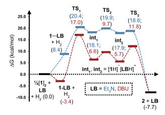
Fig. 5 Computed free energy profile for  $Et_3N$ - and DBU-assisted  $H_2$  activation with 1. Relative free energies (in kcal  $mol^{-1}$ ) are with respect to  $0.5 \cdot [1]_2 + LB + H_2$ .
