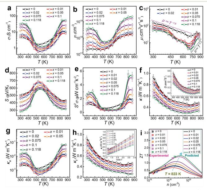
Fig. 6 Plots of measured properties of (a) T-dependent  $\sigma$ ; (b) T-dependent n; (c) T-dependent  $\mu$ ; (d) T-dependent S; (e) T-dependent S (e) T-dependent S (f) T-dependent S with inset of T-dependent S with inset of T-dependent S with predicted plots for our Cu-doped SnSe pellets.
