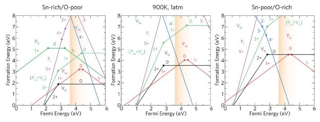
Fig. 6 The charge transition level diagrams for Sn-rich/O-poor (left), 900 K, 1 atm (middle) and Sn-poor/O-rich (right). The Fermi energy goes from the VBM (0 eV) to  $\sim$ 2.4 eV above the CBM (which is at 3.6 eV). The conduction band region is depicted by the graded orange area.
