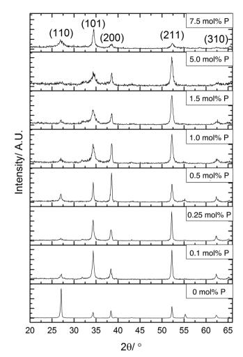
Fig. 2 X-ray diffraction patterns for  $P:SnO_2$  thin films deposited by AACVD at 550 °C. A change in preferred orientation is observed between undoped, and inclusion of phosphorus into the crystal structure.
